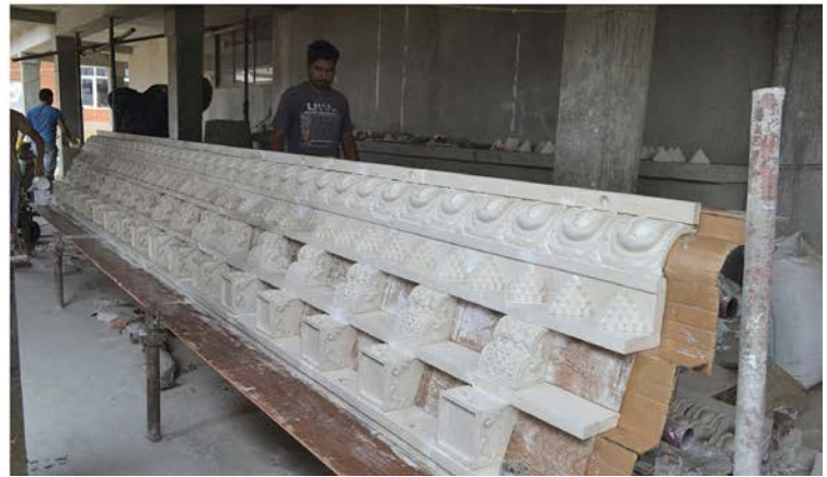
Figure 12. Array of Decorative Block Model for 2 nd Floor Interior Roof Beams Before Rubber Molding
