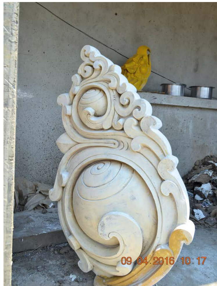
Figure 17. Model of “Pata” for Decorating Corners of 3 rd Floor Curved Roof, Before Rubber Molding
