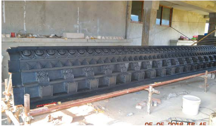
Figure 13. Same Decorative Block Model After Rubber Molding
